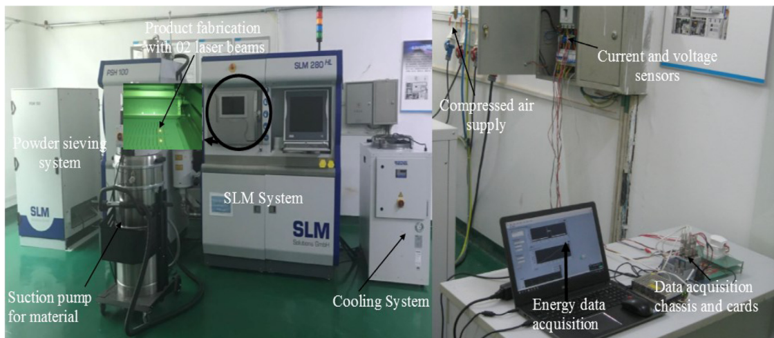
Fig. 8. Experimental system for fabrication of product and data acquisition.
